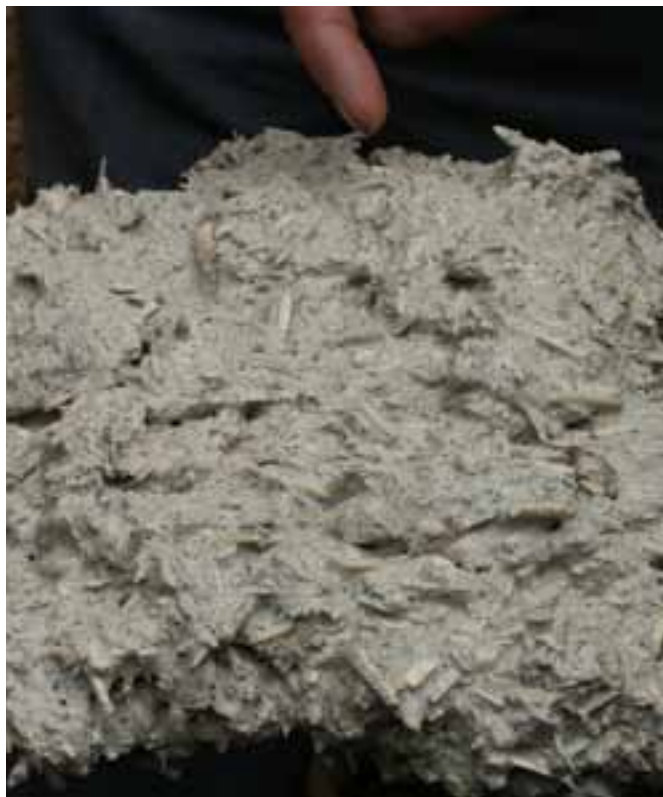
I1 Hemp-lime is a mix of chopped hemp mixed with a lime based binder. © EH/Iain McCaig
