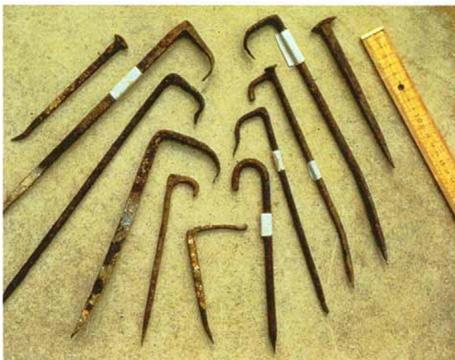
Fig 29 Selection of crooks (iron thatching hooks) from East Anglia and the Midlands. See Fig 20 for crooks in use. (Photograph copyright © John B Letts)
