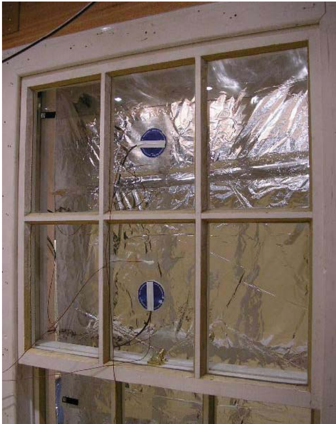
Figure 8: Low-e film on roller blind
