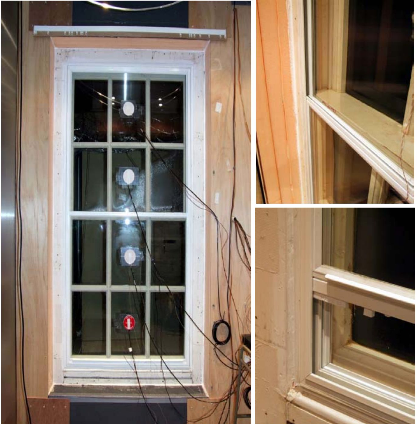
Figure 11: Secondary glazing system
