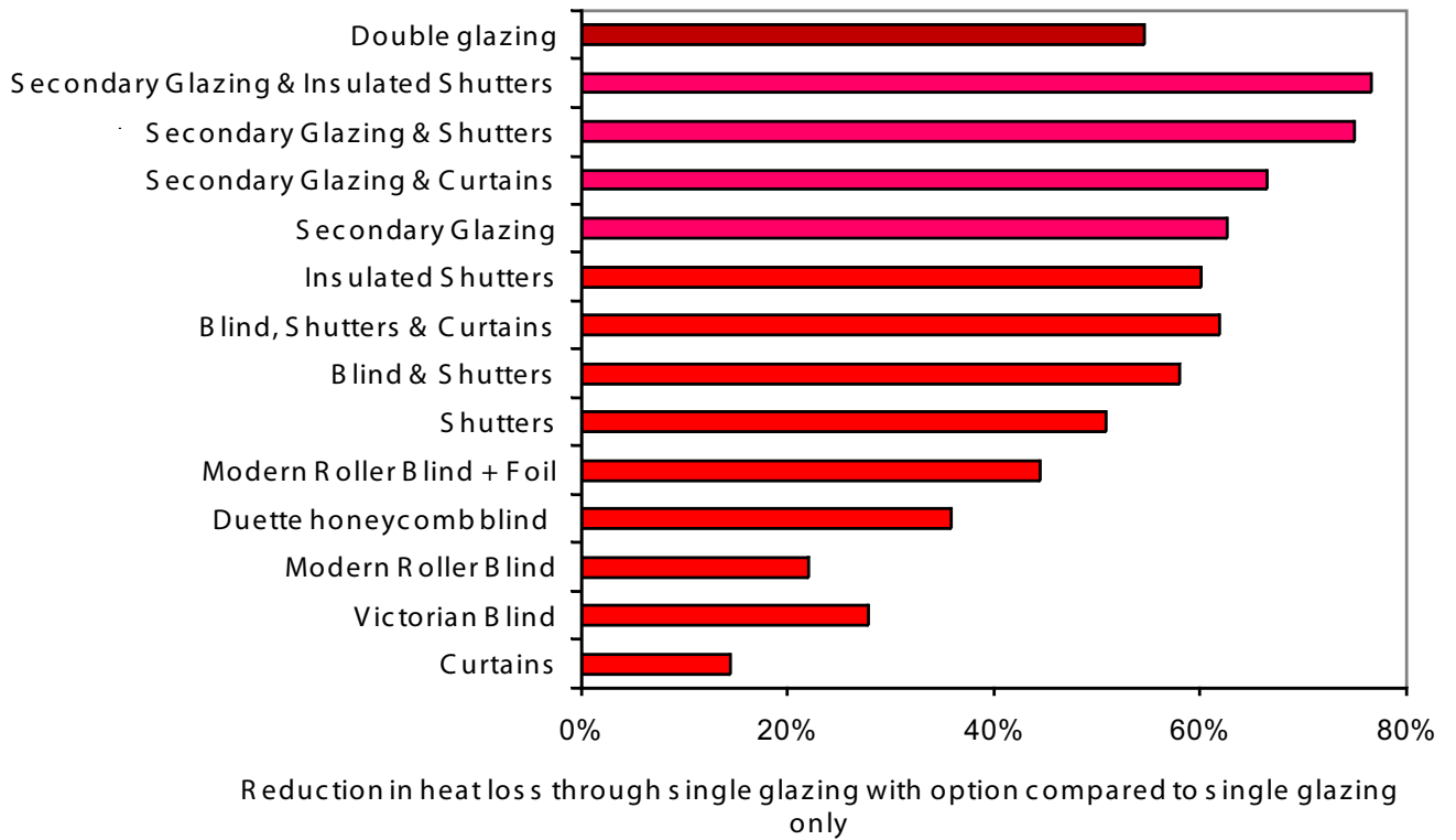
Figure 16: Effect of the options on reduction in heat loss through the glazing
