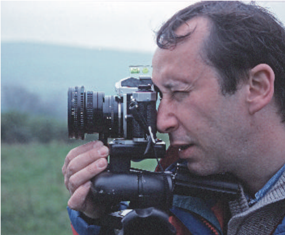
Figure 13 Conventional photographic media and equipment continue to deliver effective and economical results in a range of formats. Here a 35mm SLR camera is tripod-mounted, levelled and fitted with a rising front or 'shift' lens to minimise distortion of verticals.
